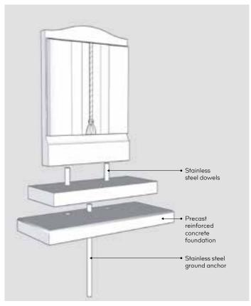
**Ground Anchor Fixing Method**
