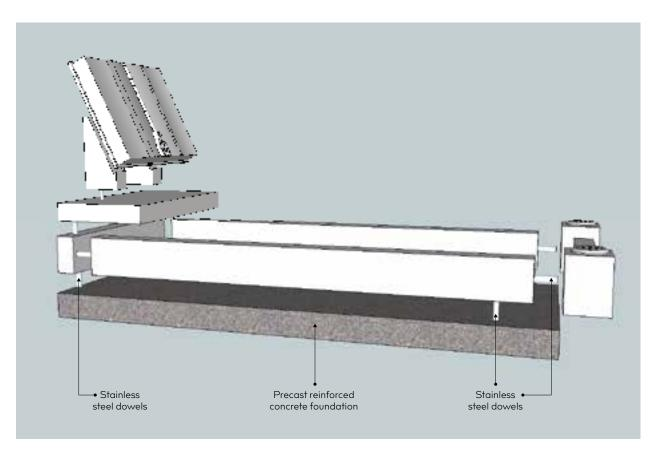
Kerb Fixing Method All sections of the memorial are securely dowelled
